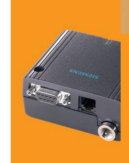
The MC35i Terminal is a robust unit with integrated GPRS and Dual-Band GSM functionality. It allows your products to immediately offer the full benefits of GPRS technology, such as permanent online connections plus cost-efficient, high-speed data transmission. The MC35i Terminal can be used with a wide range of applications, such as:
